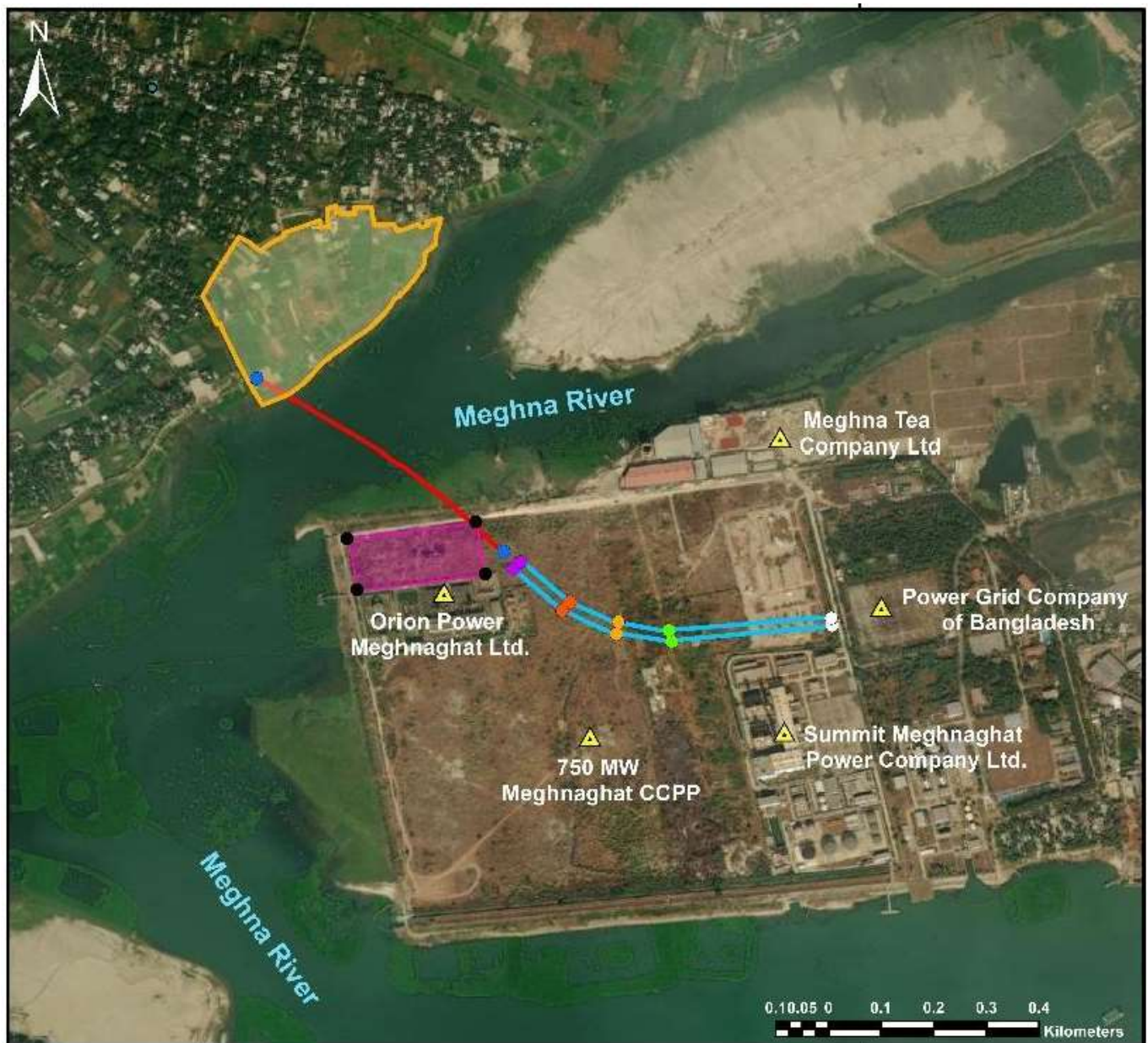
Figure 2-4: Gas Pipeline Final Route Map
