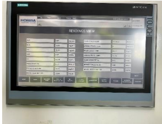
Photo 14: CEMS showing negative NO x emission value.
